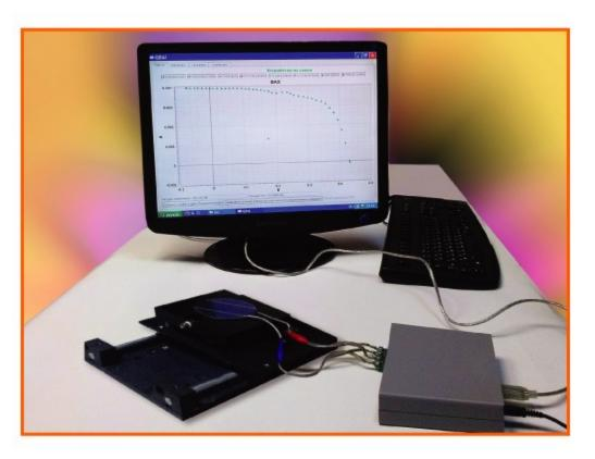
The device is designed for incremental measurement of the current through a photovoltaic cell (PVC) and voltage with automatic changing of load parameters. To improve the accuracy of measurements, the PVC is connected to the load via the current channel. The PVC voltage is measured by means of an independent circuit.
